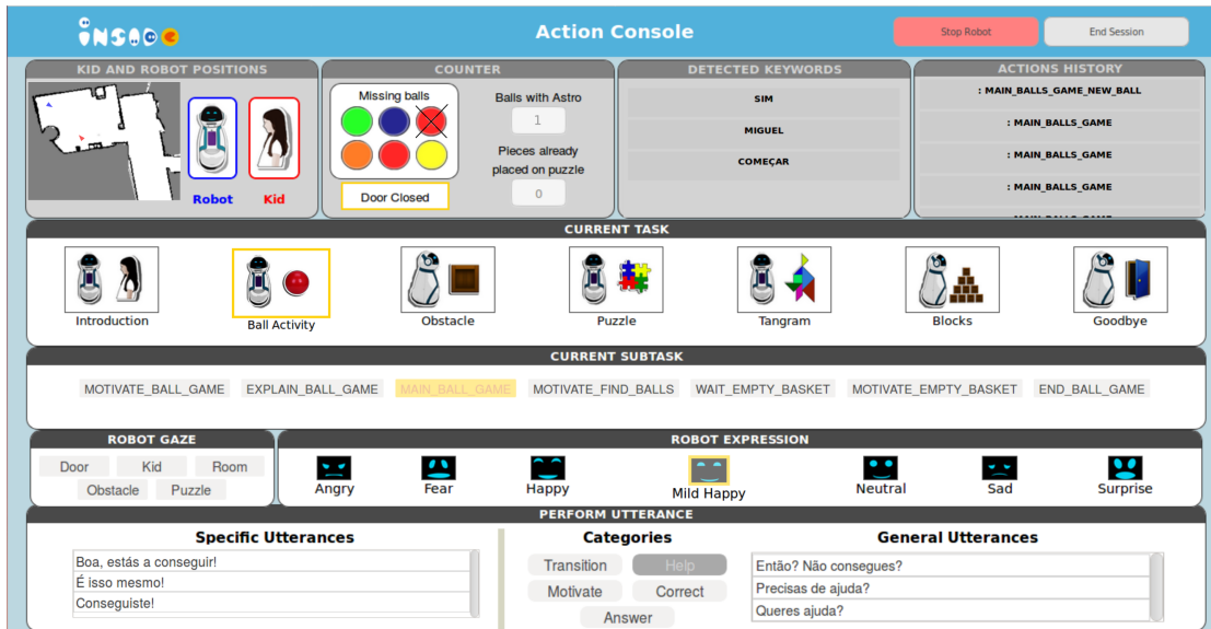
Fig. 4. Wizard-of-Oz: action console during the ball activity. The child found one of the balls and started looking for the others.
