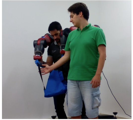
Fig. 3. Kinesthetic teaching of the intended motion: the human teacher shows the robot how to put the right strap of the backpack on a user.
