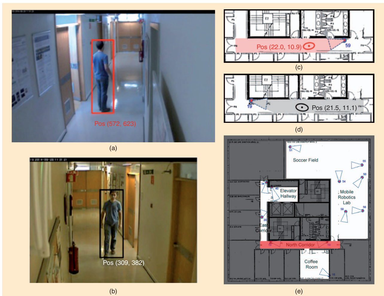
Figure 3. Our running example of a trespassing event detection: images acquired by (a) camera 59 and (b) camera 19, with detections; (c) field of view and detection of (d) camera 59 and field of view and detection of camera 19; (e) a scenario abstraction map, where the red zone corresponds to a restricted area, the white zones to accessible areas, and the dark zones to areas unsuitable for robot event attendance (e.g., cluttered zones).
